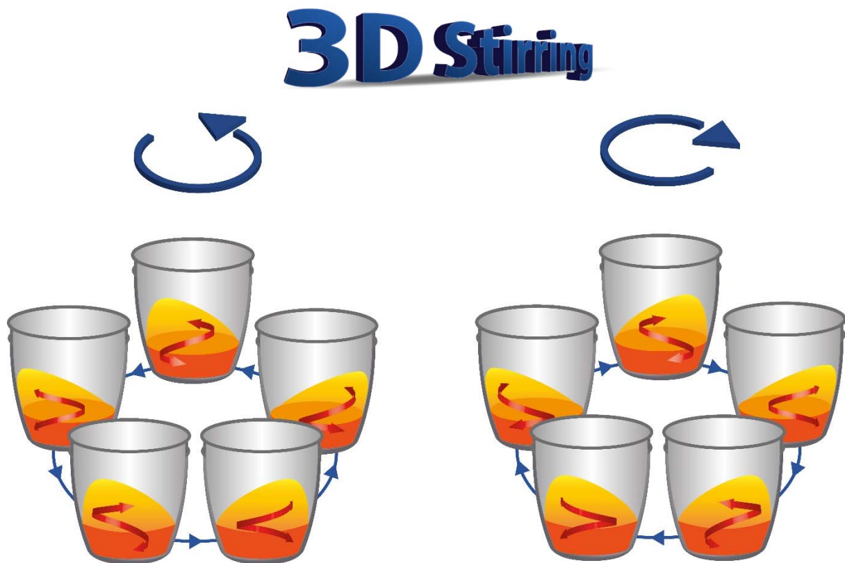
Figure 1: The principle of 3D rotation stirring in the VITRIOX machines.
