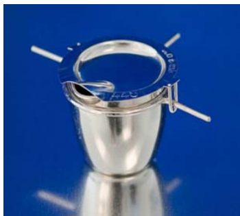
Fig. 2: Crucible for electrical fusion instrument with removable cover.
